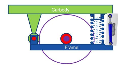
A bogie has two suspension steps, one from wheelset to frame and one from frame to carbody. The single axle running gear has only one suspension step.
