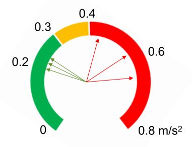
The simulations confirm that the ride comfort with passive suspension will be unacceptable.
