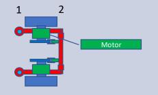
The motors on the independently rotating wheels are controlled to make the wheelset to take a radial position
